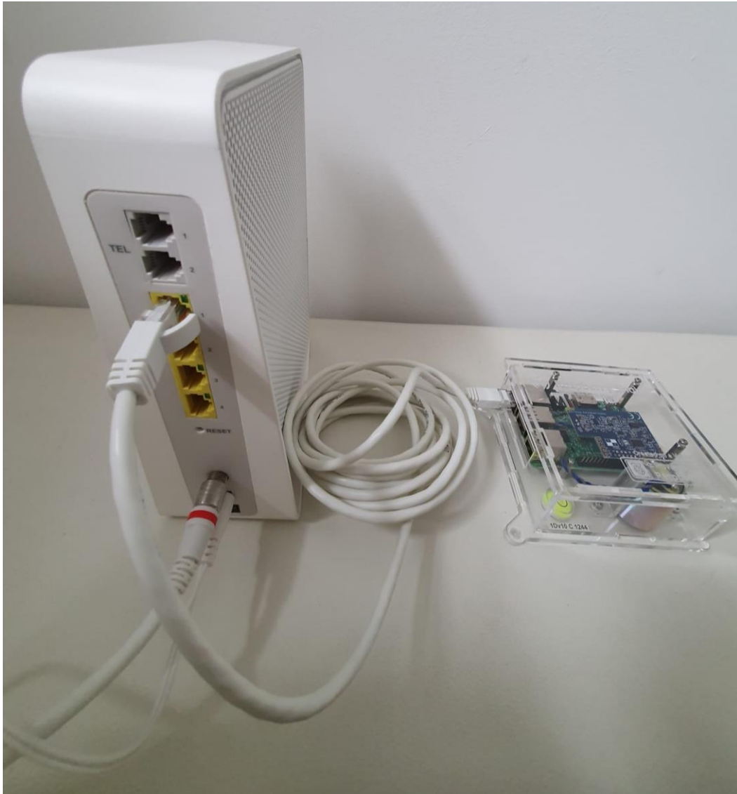
Figure 1. Shows the setup of a home internet router with the Ethernet cable plugged into the back of the router and into the side of the Raspberry Shake.
