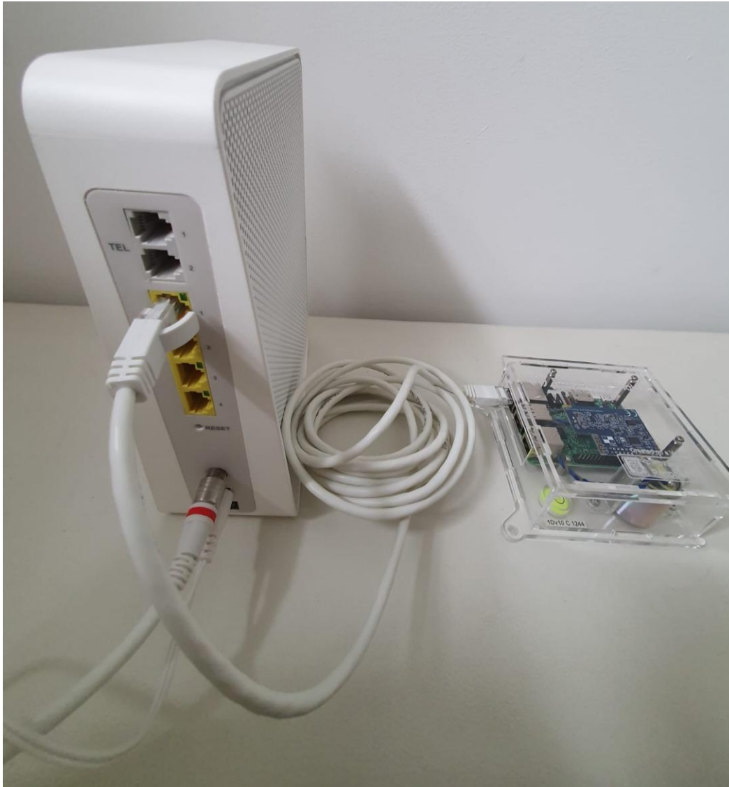
Figure 1. Shows the setup of a home internet router with the Ethernet cable plugged into the back of the router and into the side of the Raspberry Shake.
