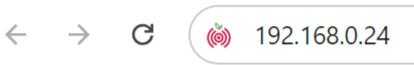
Figure 48. In an internet browser type in the IP address you obtained from Fing. Press enter.
